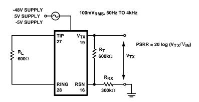
FIGURE 12. POWER SUPPLY REJECTION RATIO
