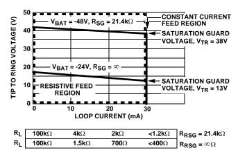
FIGURE 15. V<sub>TR</sub> vs I<sub>L</sub> and R<sub>L</sub>
