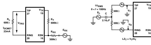
FIGURE 1. OVERLOAD LEVEL (TWO-WIRE PORT)
