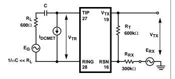
FIGURE 8. CURRENT GAIN-RSN TO METALLIC
