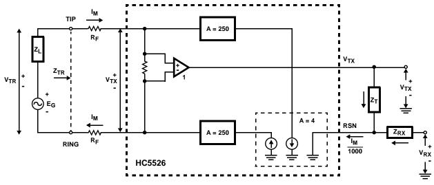
FIGURE 16. SIMPLIFIED AC TRANSMISSION CIRCUIT
